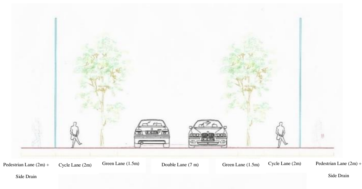
Figure 5: Two Lane Road – Cross Section
