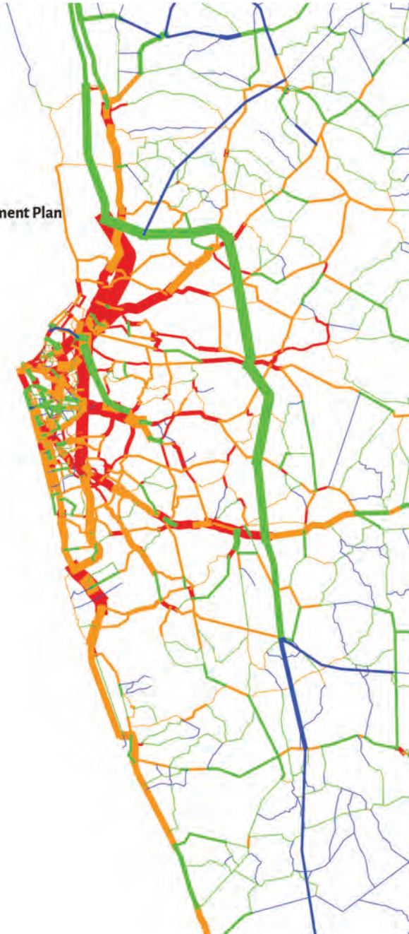
Figure 6.26: Expected Volume Capacity Ratios and Traffic Volumes (in terms of PCU) in the Do-nothing Scenario - 2035
