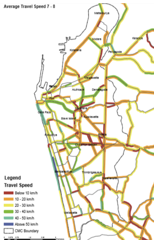
Figure 107: Average Speed during Morning Peak-hour (0700 h–0800 h) Source: CoMTrans Urban Transport Plan – 2014
