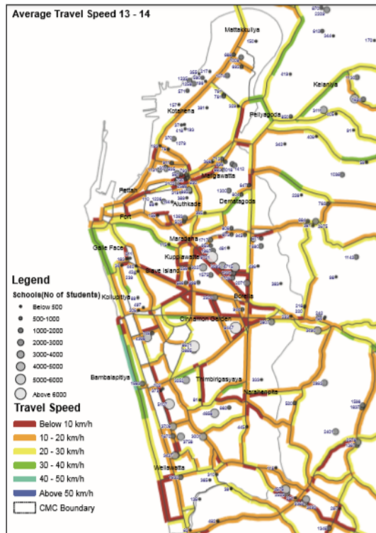
Figure 108: Average Speed during Afternoon Peak-hour (1300 h – 1400 h) Source: CoMTrans Urban Transport Plan – 2014
