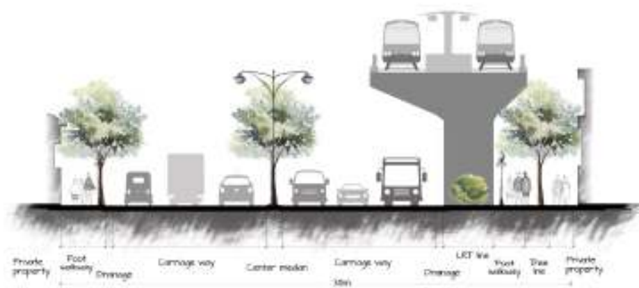
Figure 5.3: Recommended typical cross section of P1 road category with LRT Source : Western Province Division and Research & Development Unit, UDA - 2018
