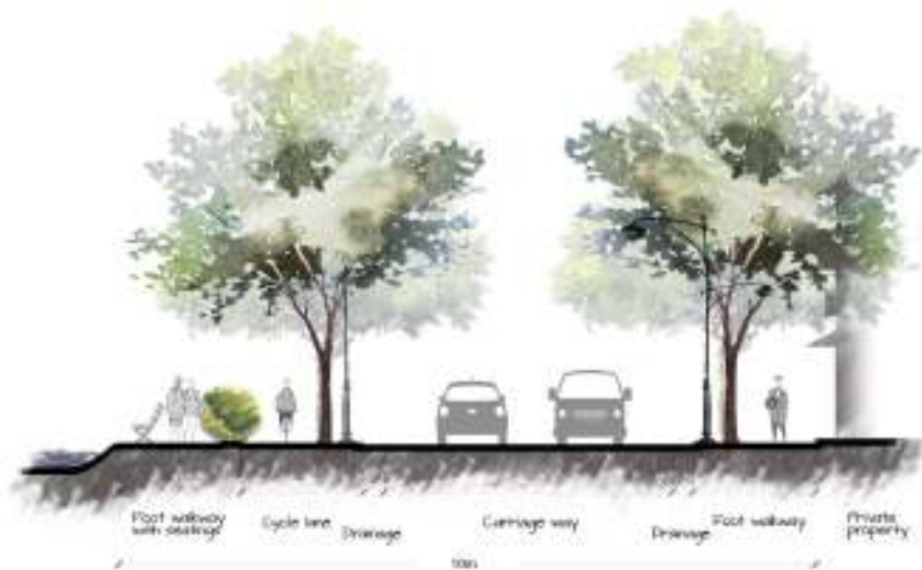
Figure 5.8: Recommended typical cross section of P6 road category Source : Western Province Division and Research & Development Unit, UDA - 2018
