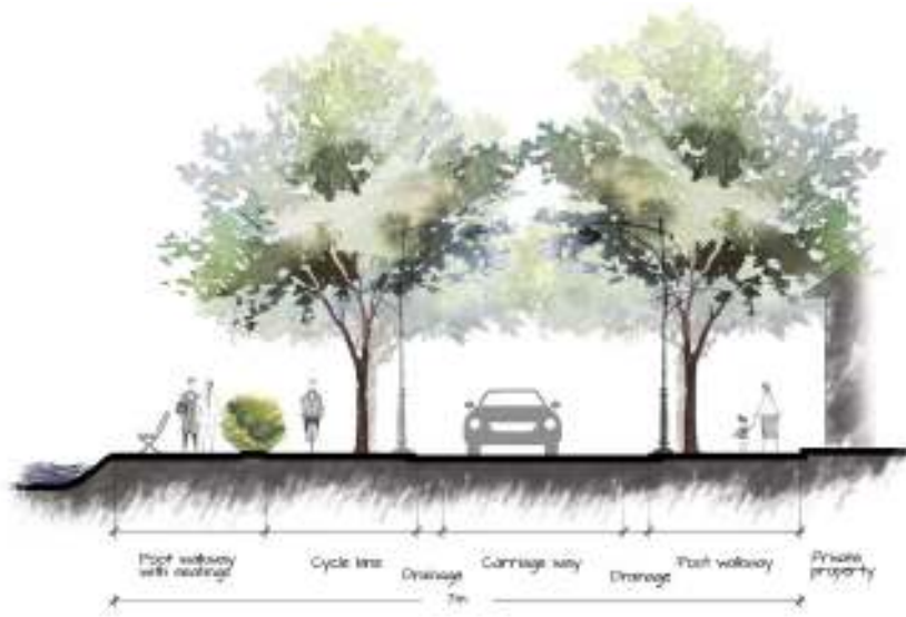
Figure 5.7: Recommended typical cross section of P5 road category Source : Western Province Division and Research & Development Unit, UDA - 2018
