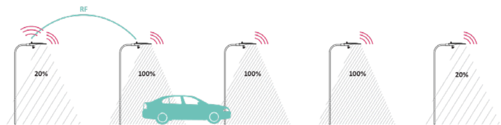
Figure No. 6.3.4.1 : Proposed Smart Street Lightning System
