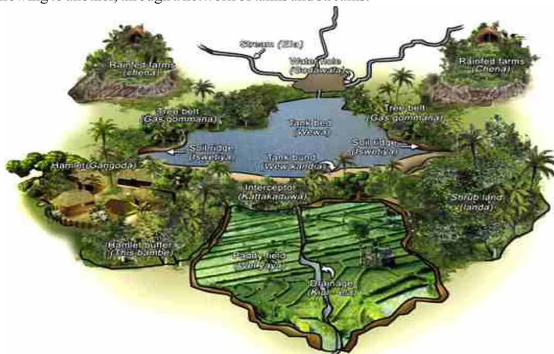
**Figure 5.2: Components and their relative positions in the small tank system in Sri Lanka**
