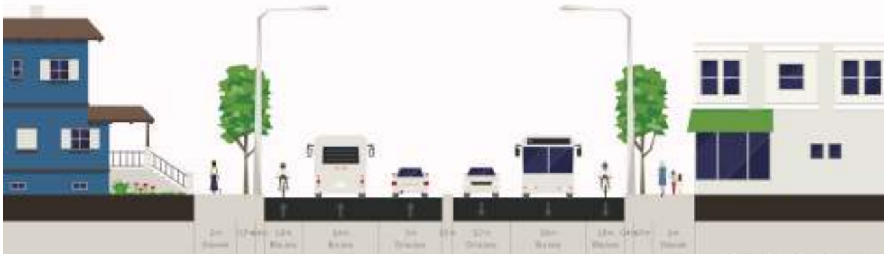
Figure 6.10 : Cross Section of P2 Roads Source : Urban Development Authority, 2021
